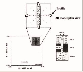
*Figure 5. Plan view and section view of the 3D model.*
