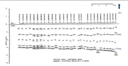
*Figure 3.* Resistivity interpretation results for one EW profile showing the conductive sediments below the trap basalts. Here, inversion was used. The small error bars indicate the 95% confidence interval and are influence in the inversion by the data errors. Well D 2 is a few km northeast from the end of the profile. The well-derived layer boundaries are indicated on the right.
