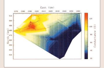
*Figure 8.* Total conductance map survey area. The Lotem stations are shown as black dots.
